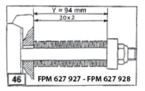
If there is a need to exceptionally modify the safety device for the user in order to adapt it to local conditions, the main principle is that the safety device spring must be adjusted in such a way as not to be activated under normal working conditions.
