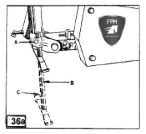
3. Move the axle (A) (figure 37), on the floating lever into the bearing for the transport position (see drawing of label B), secure it with a tightener, whereby you prevent the lever from floating.
