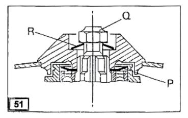
When mounting the cutting discs under the nut (Q), use a spring washer (R) for properly fastening the discs. It is always necessary to install a protective washer (P) beneath the bearing, which prevents dust and dirt from entering the cutting disc casing (figure 51).
