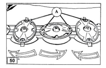
For tightening the screw (A) (figure 50) which holds the cutting blades, use a torque of 7.5 daNm.
