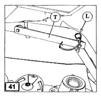
3. Using the hydraulic cylinder, lower the cutter bar into the working position.
