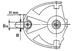
The length of the oval opening (L) on the cutting blade must not exceed 18 m
